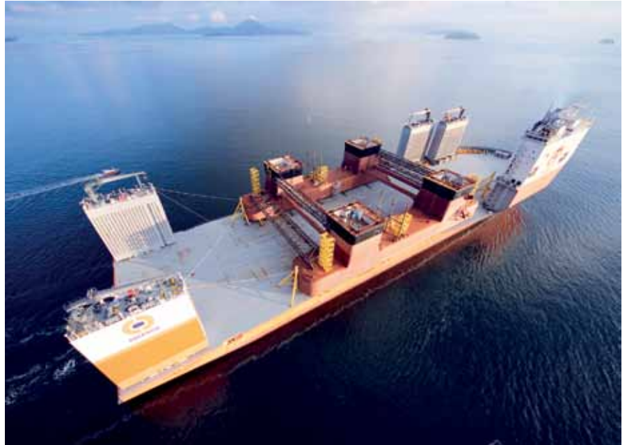
Megablocks built and assembled at BrasFELS will be fitted on the lower hull (shown above) of the first DSS™ 38E semisubmersible drilling unit that Keppel O&M is building for Brazil
